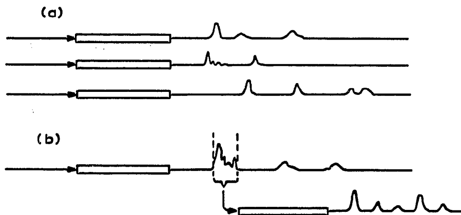
Fig. 1. Combination of GC columns, (a) in parallel; (b) in a series.
